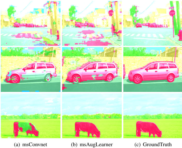
Figure 5: Raw image labeling of the multiscale ConvNet, our multiscale augmented learner and ground truth labels.
