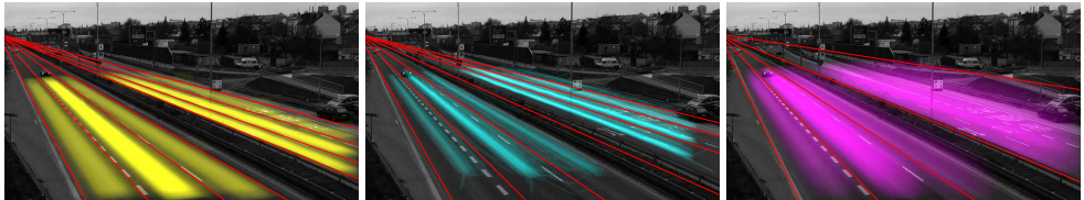
Figure 8: Traffic lane segmentation. (left) Our approach based on 3D bounding boxes. Lanes are correctly segmented even for side views. (middle) Method using trajectories of the centers of blobs [16]. (right) Method based on activity map [28].
