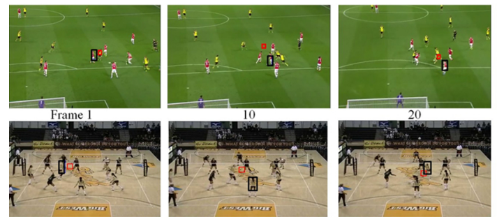
Figure 4: Behavior analysis. Red bounding boxes indicate estimated ROI, Black bounding boxes show a dominant player.
