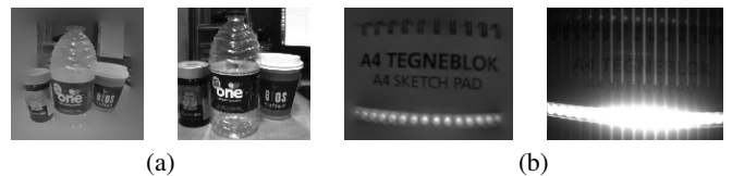
Figure 3: (a) Comparison of a reconstructed high resolution image and a down sampled normal camera image; (b) comparison of a reconstructed high dynamic range image and a normal CCD camera image.
