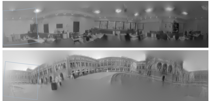
Figure 2: Spherical mosaicing for indoor and outdoor scenes. The overlaid boxes represent the field of view of the event camera.
