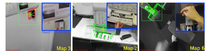
Figure 4: In the assistive mode, when a TRO is detected, video snippet is inserted showing the most relevant common MOI based on the object’s current appearance.
