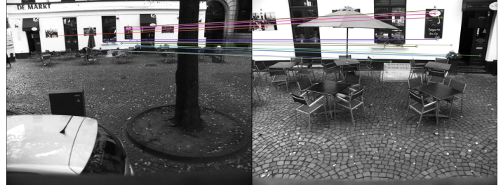
Figure 1: Illustration of cross-route image matches after pruning of false positives by means of PROSAC. Note that these are not the only correspondences found; also for other image combinations matches are tracked.
