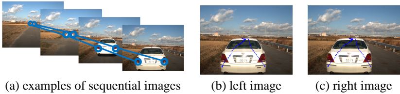
Figure 5: Real image experiment. The left and right tail lamps were used for reconstruction.
