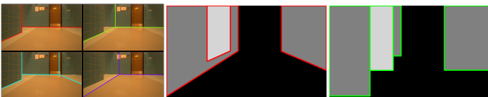
Figure 1: Example of the informative regions. (Best viewed in color.) (Left) The current set of hypotheses. (Middle) The gray-scale value reflects the informativeness I(p_j, \mathbf{M}) \in [0, 1] of each pixel p_j in the current image based on the four hypotheses. Since the hypotheses are qualitatively distinctive, the image divides into several regions based on the informativeness. (Right) Since precisely computing the exact boundary of the informative regions can be computationally expensive, we use a set of axis-aligned boxes to approximate these regions. All points within each box are set to the same I(p_j, \mathbf{M}) > 0 value (maximum informativeness among all pixels within the box), and any point that is outside the boxes has I(p_j, \mathbf{M}) = 0 .
