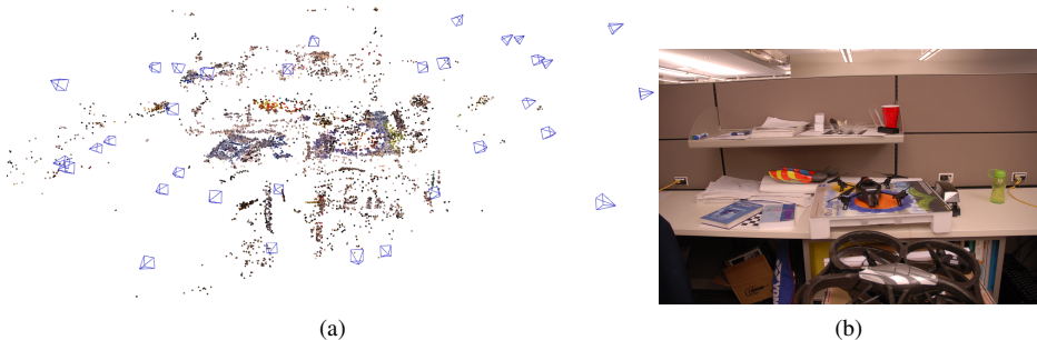
Figure 2: (a) Optimized camera poses and reconstructed structure in the cubicle dataset. (b) One of the images in a cubicle dataset.
