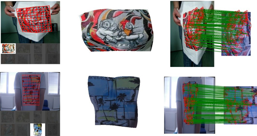
Figure 5: Reconstruction results for a single object in the image. First row: Graffiti experiment. Second row: T-Shirt experiment. Left Image: Reconstructed mesh projected in the 2D image. Middle: Reconstructed mesh in 3D. Right: Sets of clean-up matches between the target image and the object template.
