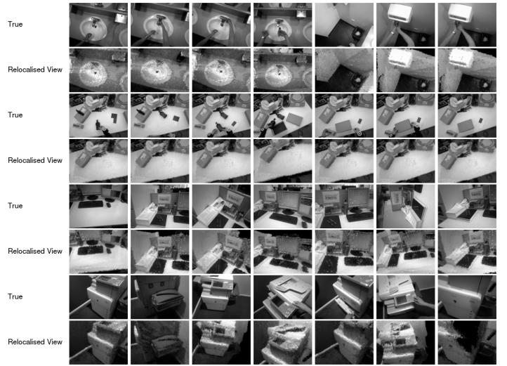
Figure 1: Examples of synthetic view regression relocalisation on four different test sequences. Images show ground-truth camera view (upper rows) and synthetic view generated from relocalised pose (lower rows).
