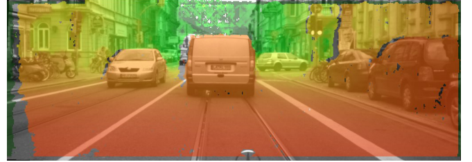
(a) Dense SGM Stereo reconstruction [1]. The color represents the distance to the obstacle with red being close and green far away.
