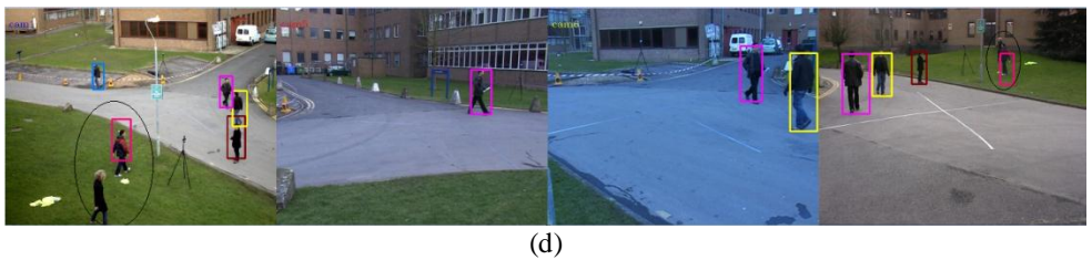
Figure 5. Some detection results on PETS09 S2L1 and APIDIS datasets. (a) Sample detection result on the PETS09 S2L1 dataset. (b) and (c) An example for the foreground information and detection results on the APIDIS dataset. (d) A failure case due to the presence of the slope (black circle in view 1 and view 8).
