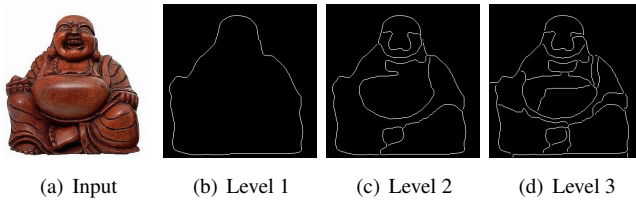
Figure 2: Segmentation hierarchy. Image of a laughing Buddha shown in (a), and three levels of the corresponding segmentation hierarchy in (b), (c), (d).
