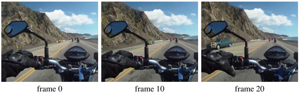
Figure 1: Example sequence with overlaid box showing the output of our specialized “forward” motion model, where the velocity and scale of objects approaching the camera tend to increase. Neither Brownian nor constant-velocity motion models are as successful at tracking interest points here.
