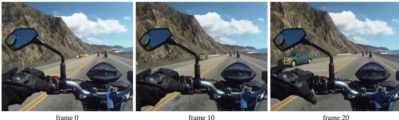
Figure 1: Example sequence with overlaid box showing the output of our specialized “forward” motion model, where the velocity and scale of objects approaching the camera tend to increase. Neither Brownian nor constant-velocity motion models are as successful at tracking interest points here.
