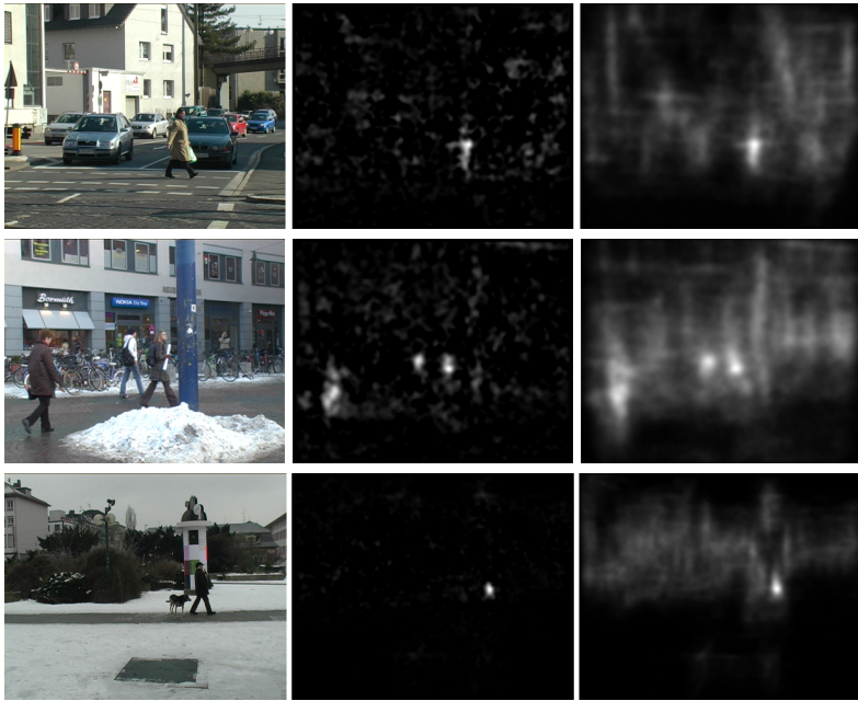
Figure 3: Hough maps for example test images (left) from the TUD pedestrian dataset, with discriminative weights (middle) and standard uniform weights (right). Note how in the case of discriminative voting correct detection peaks are clearly pronounced while background noise is significantly reduced.
