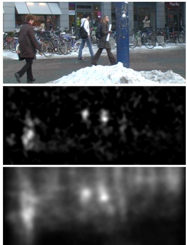
Figure 2: Hough maps for an example test image from the TUD pedestrian dataset (top), with discriminative (middle) and uniform (bottom) weights
