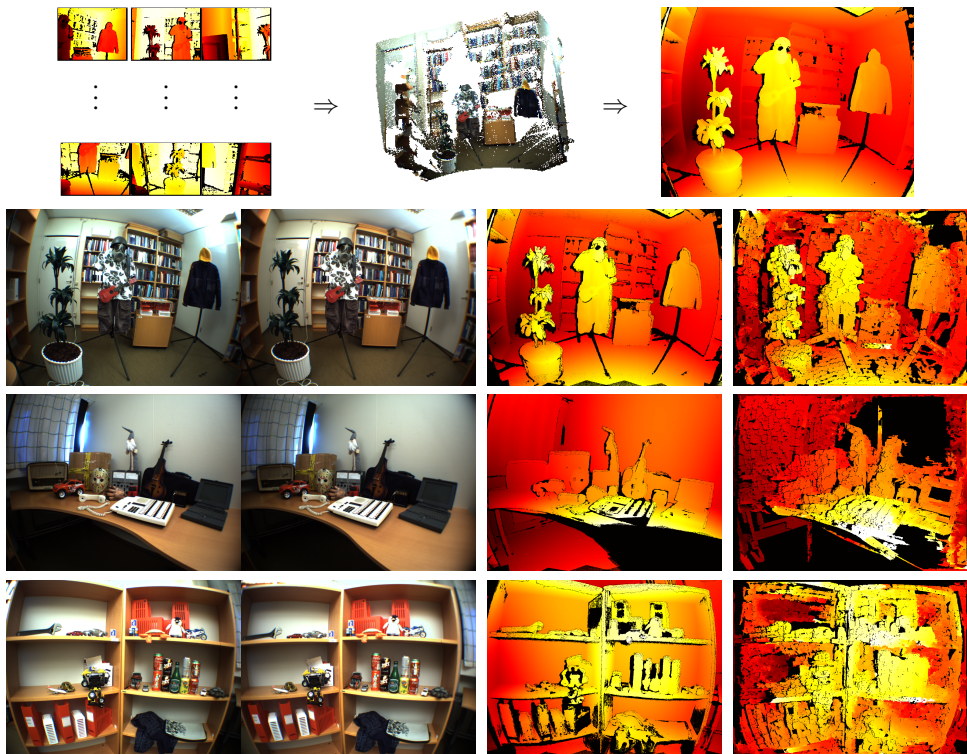
Figure 2: Top: Example of ground-truth generation. Left: Individual Kinect range scans. Centre: several range scans projected into 3D. Right: The magnitude of the fused ground-truth disparity map.
