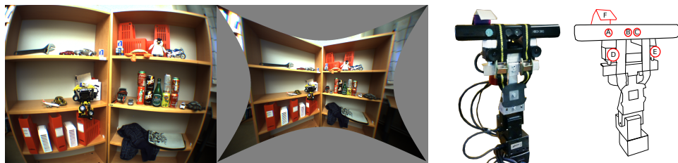
Figure 1: Left: In wide-angle images, angular resolution is near uniform. If they are rectified to preserve straight lines [14], most of the image is spent representing the periphery. Right: Pan-tilt stereo rig with Kinect. (A) - SLP projector, (B) - RGB camera, (C) - NIR camera, (D) - Left wide-angle camera, (E) - Right wide-angle camera, (F) - Diffusor (raised).
