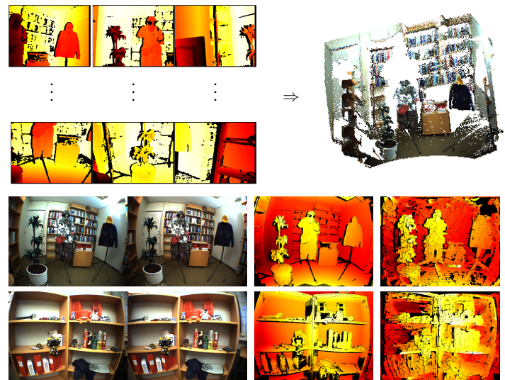
Figure 2: Top: Example of ground-truth generation. Left: Individual Kinect range scans. Right: several range scans projected into 3D. Bottom: Examples of views for two scenes. Columns left to right: Left wide-angle image, right wide-angle image, magnitude of disparities deemed reliably reconstructed. The final column shows magnitude of disparity estimate obtained using tuned CtF-BFP.
