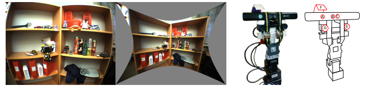
Figure 1: Left: In wide-angle images, angular resolution is near uniform. Middle: If they are rectified to preserve straight lines, most of the image is spent representing the periphery. Right: Pan-tilt stereo rig with Kinect. (A) - SLP projector, (B) - RGB camera, (C) - NIR camera, (D) - Left wide-angle camera, (E) - Right wide-angle camera, (F) - Diffusor (raised).
