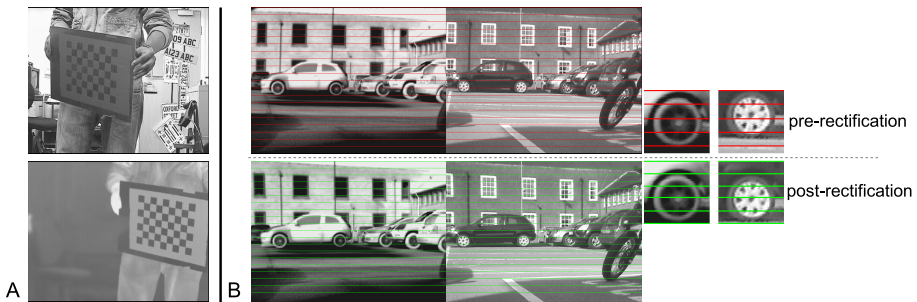
Figure 1: Cross-spectral calibration target (A) and rectified result (B)
