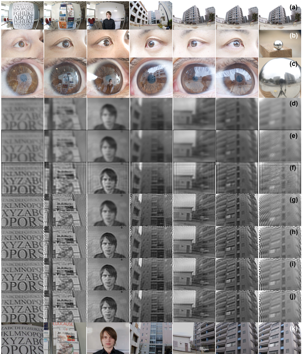
Figure 6: SR result for different scenes (from datasets of 10 eye/mirror images). (a) Scene images taken from the same position as the eyes, using a fisheye lens. (b) Single original image. (c) Cropped eye region. (d)-(g) Local plane projection of recovered environment map at region of interest: (d) Single LR image, natural neighbor interpolated. (e) Combined aligned LR images, natural neighbor interpolated. (f) Blind deconvolution of (e). (g)-j) SR result: (g) ML, before convergence. (h) MAP using LoG, (i) BL and (j) BTV prior, after convergence. (k) Cropped pictures of the region of interest from scene images in (a). (right column) Result from a spherical mirror at the size of the human cornea.
