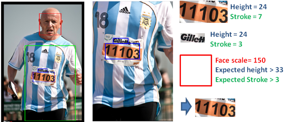
Figure 6: Tag Selection: (a) The tag is searched in the green bounding box; (b) two tags are detected – marked in blue. (c) the face scale is used to limit the size and stroke of the tag, and filter out wrong candidates.
