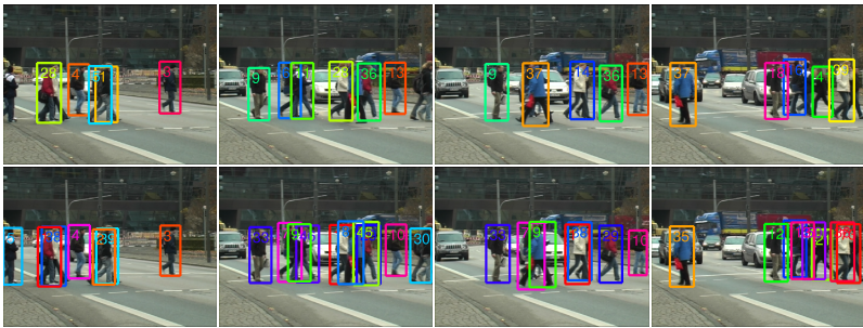
Figure 7: Tracking-by-detection results on the TUD-Crossing dataset with single-person detector (top row) and our joint detector (bottom row). Colors and numbers indicate tracks corresponding to different people.
