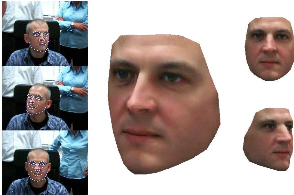
Figure 8: The reconstruction of a real-life head. The three views were chosen automatically from a short video sequence captured using a webcam.
