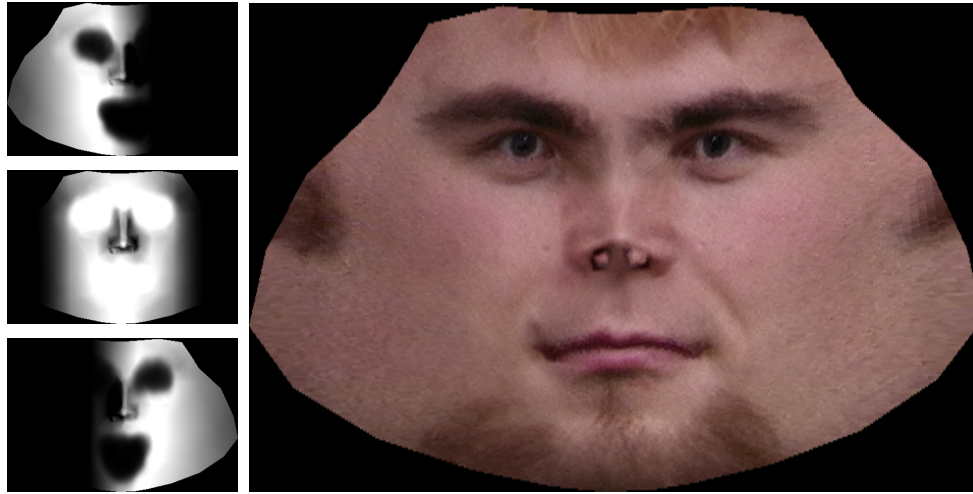
Figure 6: The left most images show the weightings, W_k , used when combining texture maps from multiple views. The right image shows one such merged texture map, T .
