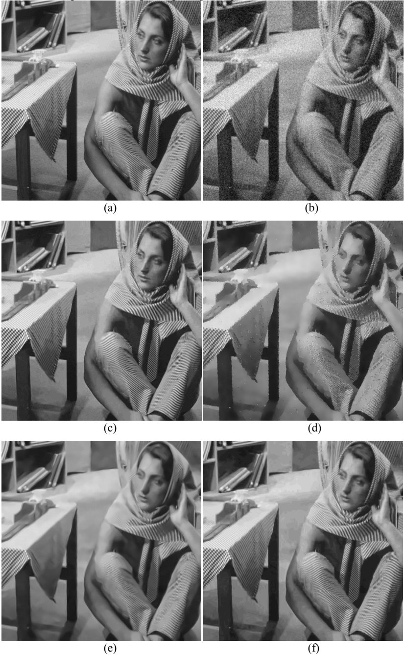
Figure 4: (a) A noise-free Barbara image; (b) The noisy image with AWGN of a Std \sigma_n=25 ; (c)–(f) Denoised results by FP-NAD, PM,SAFIR and BM3D, respectively.
