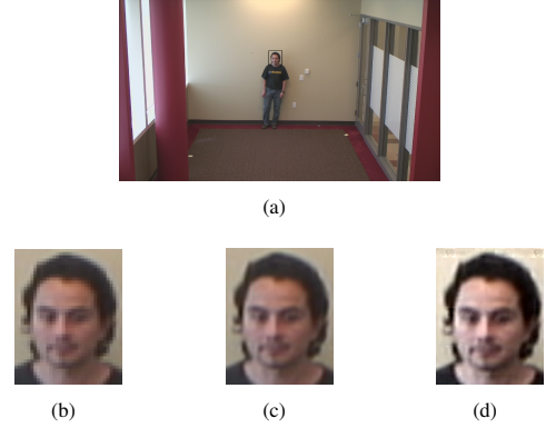
Figure 2: Illustration of the surveillance camera output and the SR output. (a) Depiction of a frame acquired by surveillance camera (the black bounding box output indicates successful face detection), (b) magnification of the area in the bounding box (IPD \approx 11 pixels), (c) output of BCI, and (d) output of the proposed (UHSR) algorithm.
