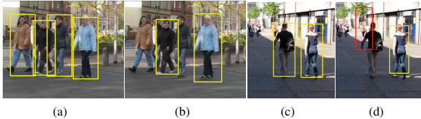
Figure 1: Performance of our detector without (b,d) and with (a,c) complementary shape information
