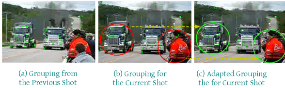
Figure 3: Effect of adaptive grouping. Green labels imposed on image indicate to which group the point belongs. (a) Grouping from the previous shot, (b) Grouping for the current shot without taking information from the previous shot and (c) Grouping for the current shot with information from the previous shot. Regions in red ellipses in image (b) indicate incorrectly clustered points compared to image (a). Corresponding regions in image (c) indicate improvement over the previous grouping.
