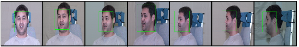
Figure 1: Opencv frontal and profile face detector results
