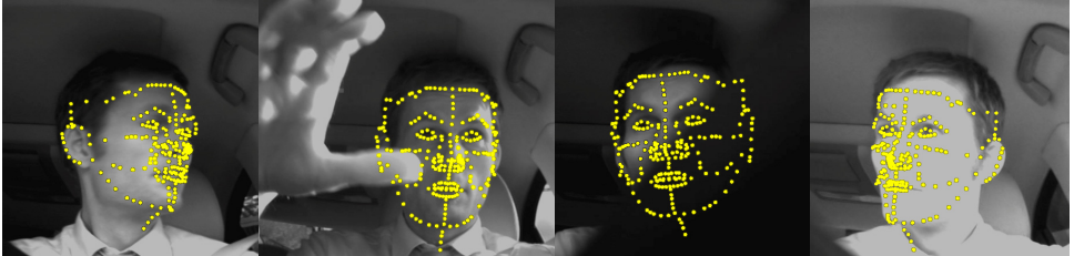
Figure 1: Search results. The example frames from in-car videos show many problems including: occlusion; a non-uniform background; variable illumination; low contrast; and extreme pose.
