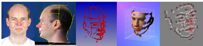
Figure 1: The model is built using manual markups. Each subject is marked in front and profile to create a 3D point set. A mesh is warped to match each subject and a subset of vertices on features of interest is extracted from each mesh. View-based patches are used to search.
