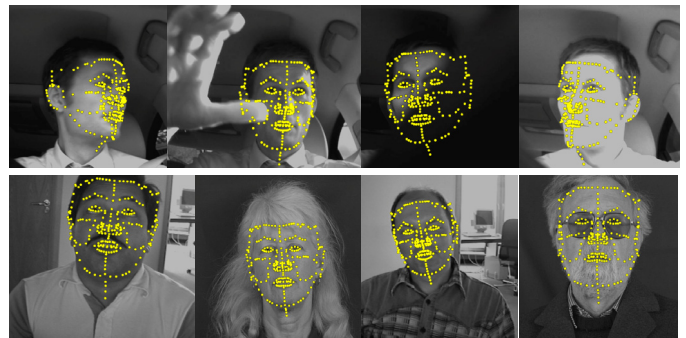
Figure 2: Search results. These example images from in-car videos and datasets show many problems including: occlusion; a non-uniform background; variable illumination; low contrast; extreme pose; glasses; and facial hair.
