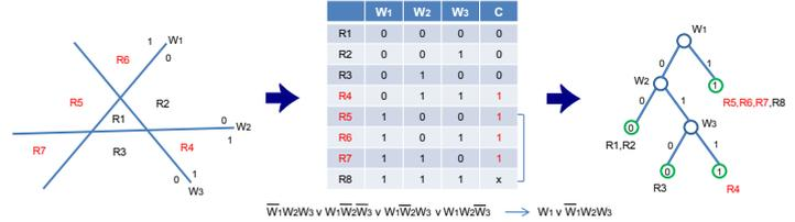
Figure 3: **Boolean expression minimisation for an optimally short tree.** (a) A boosting classifier splits a space by binary weak learners (left). The regions are represented by the boolean table and the boolean expression is minimised (middle). An optimal short tree is built on the minimum expression (right).
