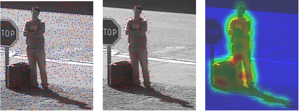
Figure 2: Left: Union of keypoints detected on background and current image. Blue keypoints are detected on both images while the red ones are detected on only one image. Center: Non matching keypoints between the background image and the current view. Right: The associated density probability function. Blue is for low, green for medium and red for high density values.
