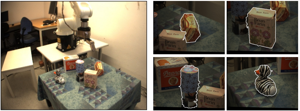
Figure 1: A wide field view in which object hypotheses are searched using attention (left) and segmentations of each found hypothesis in the foveated view (right).
