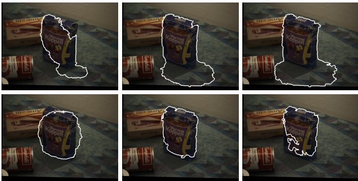
Figure 4: The 1st, 5th and 10th updates of a segmented box, without a flat surface model (upper) and without disparities altogether (lower).
