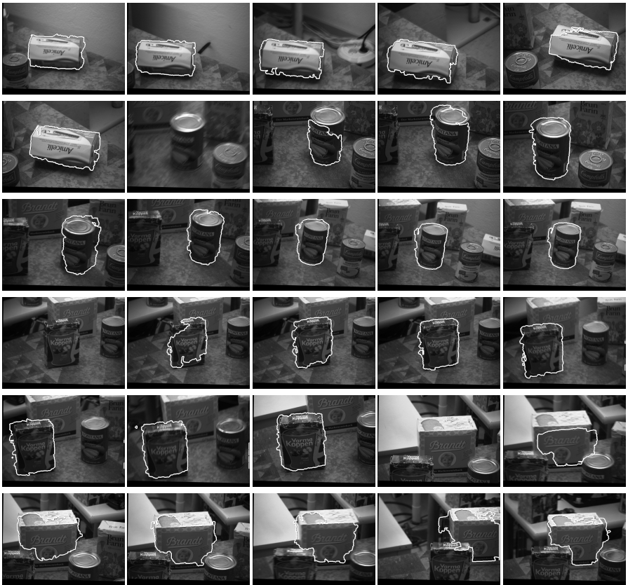
Figure 7: Sequence of segmentations obtained using the proposed system, while tracking objects of interest detected by an attention system. With the system running in around 8 Hz, the delay between each images is about a second.
