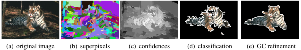
Figure 1: Summary of our approach. First the input image in (a) is segmented into superpixels, shown (b). Then the trained classifier is applied to each superpixel individually, classifier confidences are in (c). Based on confidences, superpixels are classified into salient/background, shown in (d). Finally the results in (d) are refined with graph-cut optimization, and the result after the refinement is in (e).
