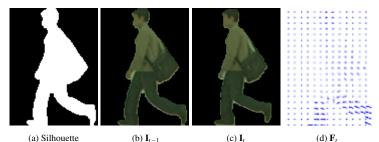
Figure 1: Computing figure-centric optical flow field. (a) shows the silhouette at frame t-1; (b)&(c) are the extracted figure-centric images of the walking person at t-1 and t respectively; (d) is the computed optical flow field.
