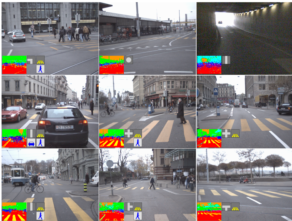
Figure 5: Example images from a 30-minute sequence, Seq. DAY. For each image, the bottom left shows the patch classification output, as well as the scene classification (road type, present objects). Result video available at http://www.vision.ee.ethz.ch/~aess/ . Figure is best viewed in color.
