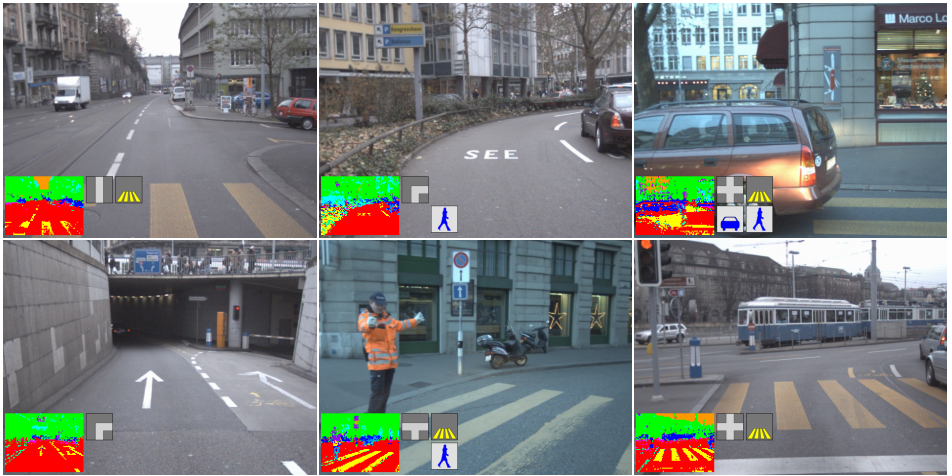
Figure 7: Typical failure cases (from left to right, top to bottom): incoming junctions are ignored due to low resolution; patch classifier mistakes car for pedestrian; headlight’s reflectance confuses the patch classifier; sidewalk is difficult to distinguish from road; road geometry not in set of classes; too complicated/ambiguous road geometry.
