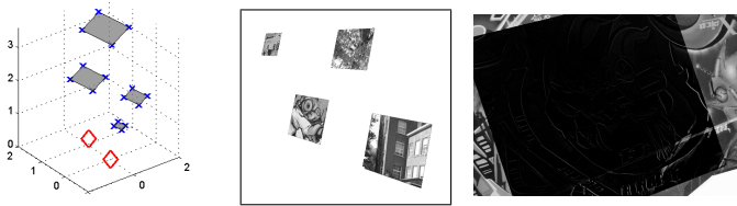
Figure 5: Bundle adjustment: (left) artificial setup for bundle adjustment, (middle) example image for one camera position; Homography estimation: (right) overlay of images using the homography estimated with covariances.
