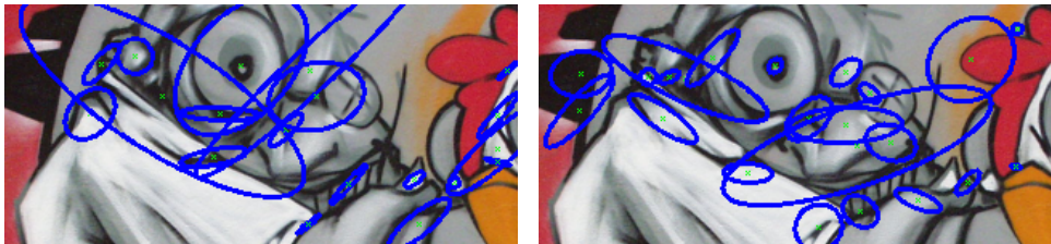
Figure 1: Covariance estimates for interest regions detected by SIFT (left) and SURF (right).
