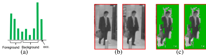
Figure 8: (a) Histogram of relative disparities. (b) A pair of ROIs. (c) Its foreground regions.
