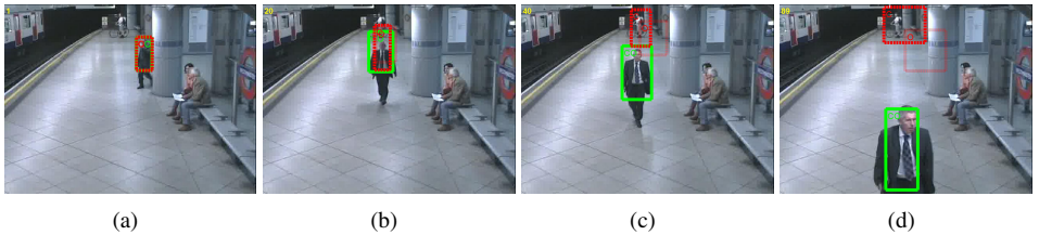
Figure 3: Importance of fusion for adaptive tracking. Adaptive color only (dashed red), orientation only (dotted red), and fused tracking (solid green; same as Figure 2(q-t))
