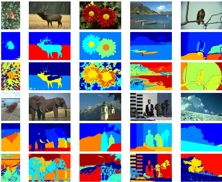
Figure 3: This figure compares the output of the automated segmentation procedure to human labeled segmentations. The first and fourth rows contain the input imagery, the second and fifth rows contain human segmentations while the third and sixth rows contain machine segmentations.
