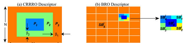
Figure 2: Partition of a group image by two descriptors. Left: the Center Rectangular Ring Ratio-Occurrence Descriptor ( \beta_1 = M/2\ell, \beta_2 = N/2\ell, \ell = 3 ); Right: the Block based Ratio-Occurrence Descriptor ( \gamma = 1 ), where white lines are to show the grids of the image.
