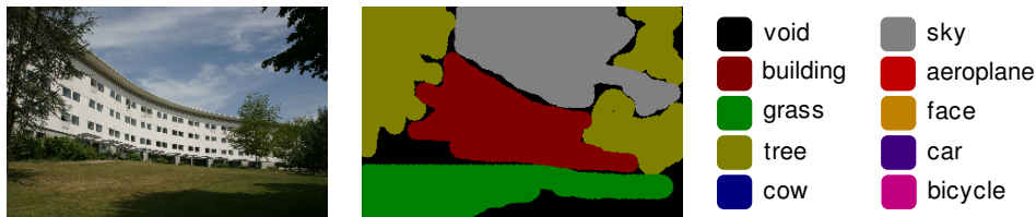
Figure 1: Semantic segmentation example for an image from the MSRC database. The legend specifies the different categories used in the paper.
