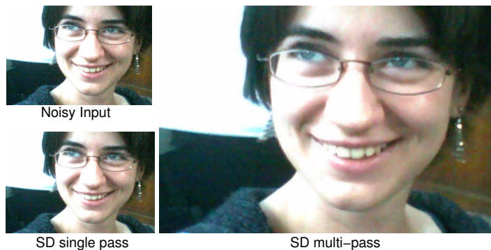
Figure 2: Single and multi-pass stochastic denoising results on a noisy image taken with a cell phone camera. The multi-pass denoising algorithm yields improved noise removal in this case, removing noise correlated over small pixel neighbourhoods while preserving sharp boundaries
