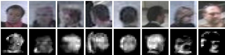
Figure 4: Examples of head image feature descriptors (bottom row) constructed from input images (top row) by selecting the maximum KL divergence \delta_{KL} between each input image and multiple pose mean templates for each pixel position.
