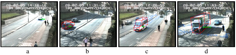
Figure 6 Four examples generated with 3DHOG. a) Missed car due to low contrast of the vehicle bonnet and roof. b) Misclassified SUV as van due to similar size and appearance. c,d) Correct detections, the blue outline indicates the foreground mask. Due to the auto-iris function of the camera, the mask is too large for the large white vehicles. The 3DHOG classifier can correctly locate and classify the vehicles because it does not rely on the foreground mask.
