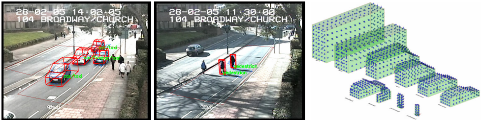
Figure 1 Example views from the i-LIDS dataset with detected and classified pedestrians and vehicles. The image on the right illustrates the 3D models used.
