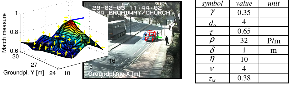
Figure 4 Left: Example of car detection with occlusion of pedestrians showing match measure surface with a good peak. Right: Parameters used during evaluation.
