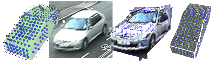
Figure 2 Extraction pipeline: One 3D model with interest points \mathbf{P} followed by input image I , extracted image patches \mathbf{I}_p and feature vectors \hat{\mathbf{f}}_k . The radius of cones indicates the weight q_j of point \mathbf{p}_j .
