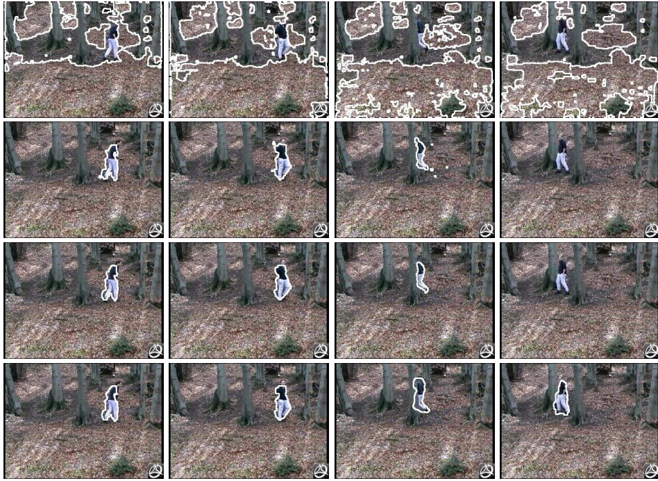
Figure 2: Tracking results for person walking in busy background: (top row) region competition (7) without shape, (2nd row) fixed photometric model (5) without shape, i.e. m^\gamma = m^{\gamma=1} ; (3rd row) as last row but with shape prior ( \lambda_\psi \neq 0 ), (final row) as last row but updating the photometric model from frame to frame, i.e. m^\gamma \neq m^{\gamma=1} . Data from [11].
