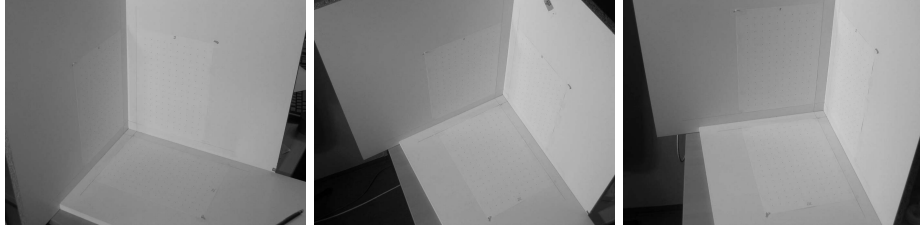
Figure 1: The three camera views. The camera centers are approximately 1.3 m from the corner and approximately 0.5 m apart. Each plane is covered with a calibration patten of 10 \times 15 small dots, approximately 18 mm between the rows and columns.
